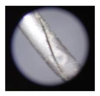
Figure 4.4: broken capillary of the  $^3He$  impedance
