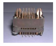
Figure 3.3: side view of the socket after milling
