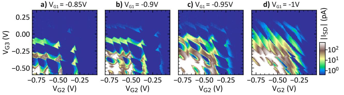
Fig. S3. Charge stability diagrams for different values of voltage applied to the central nanogate G1. By decreasing  $V_{G1}$  the inter-dot tunnel coupling is increased, as evident from the transition from a double quantum dot (a) to a more single-dot-like configuration (d). Data were taken at  $V_{SD} = -5$  mV and  $V_{L1,L2} = -4.5$  V.
