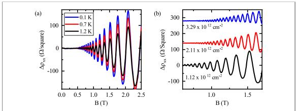
**Figure B1.** SdH oscillations. (a) We can extract the effective mass by analysing the temperature dependent SdH oscillations at various magnetic field values B. (b) The envelope of the SdH oscillations in the fully spin and valley degenerate regime (< 2.5 T) we can extract the quantum lifetime  $\tau_q$  for various densities. Curves are offset for clarity.
