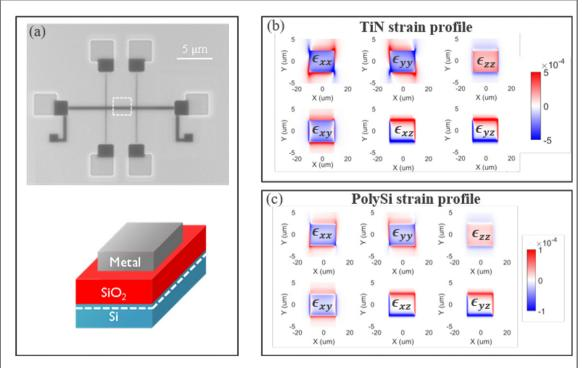
**Figure D1.** Gate material strain simulations. (a) Schematic of the Hall bar used for the strain simulation. The strain in the channel was calculated using sprocess in the region indicated by the dashed white line. (b) and (c) The strain in the channel for the polySi and TiN respectively. The model uses literature values for the thermal expansion coefficient for both materials.
