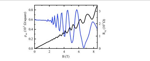
**Figure C1.** TiN data at high fields. Longitudinal resistivity  $\rho_{xx}$  (blue) and transverse Hall resistance  $R_{xy}$  (black) of the sample measured with a TiN top gate at 500 mK. Both the not well developed zeroes in  $\rho_{xx}$  and the oscillating  $R_{xy}$  indicate multiple subband occupancy.
