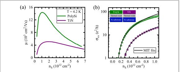
**Figure 3.** Gate material study. (a) The channel mobility  $\mu$  with respect to sheet density  $n_S$  for polySi (green) and TiN (violet), both at 4.2 K. The mobility shows a decrease by a factor of three when changing the top gate material from polySi to TiN. (b) Longitudinal conductivity  $\sigma_{xx}$  with respect to sheet density. The fits to percolation theory (black) show a significant difference between the polySi and TiN percolation densities.
