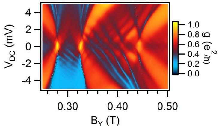
Left: schematic of the device structure. Dark blue represents the 1D wires, quantum Hall edge states are depicted in purple. Local top gate (green) controls the electron density and can be used to tune the system into the tunneling configuration regime. Right: Tunneling conductance as a function of magnetic field (horizontal axis) and bias voltage (vertical axis).
