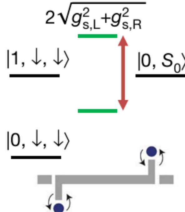
when both spins are simultaneously tuned into resonance with the cavity, the excited-state spectrum splits into dark state given here by spin triplet state and two bright states.
