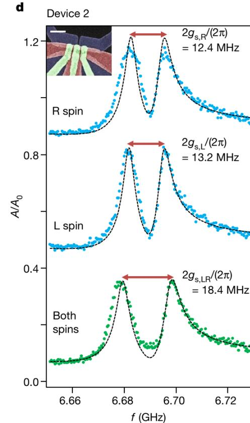
For N identical spins, Jaynes-Cummings model predicts a collective  $\sqrt{N}$  enhancement of the coupling rate
