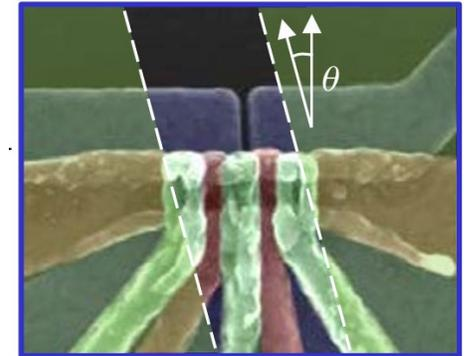
To overcome this local difference in the magnetic field, they tilted the micromagnet by  $15^\circ$  Angle,  $\phi$  as an additional degree of freedom.
