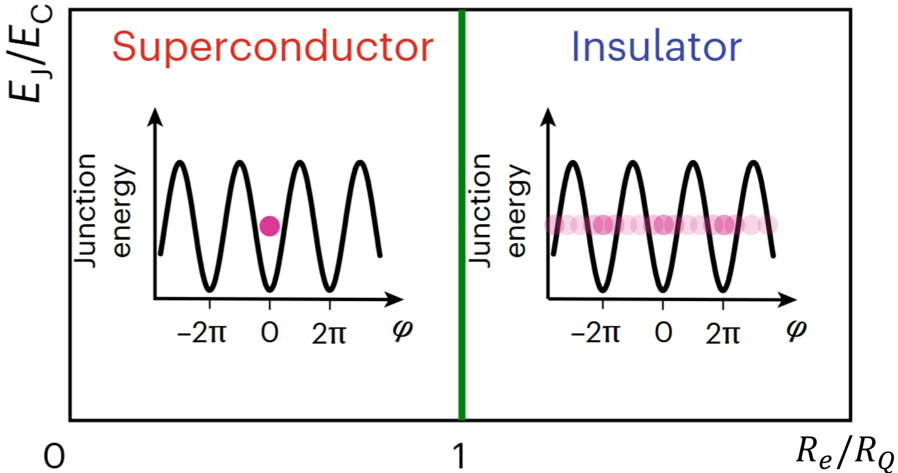
High  $R_e$  induces voltage noise which couples to the superconducting phase
