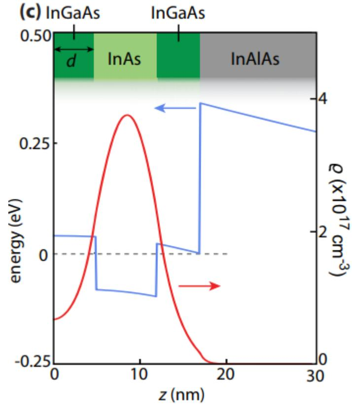
Calculated charge distribution for  $d = 5$  nm
