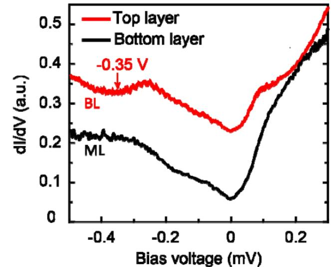
Figure S4| Layer-dependent tunneling spectra of as-grown epitaxial graphene
