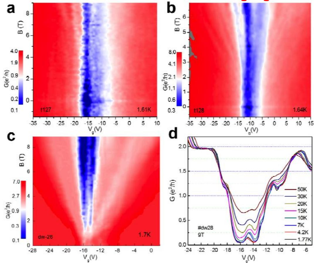
Figure S2| Magneto-transport measurements of other Z-GNR devices. **a**, sample# t127,  $l \sim 525$  nm,  $w \sim 60$  nm. **b**, sample#t128,  $l \sim 471$  nm,  $w \sim 101$  nm. **c**, sample#dw-28,  $l \sim 500$  nm,  $w \sim 120$  nm. **d**, Temperature-dependent magneto-transport measurement of sample#dw-28 at  $B=9$  T.
