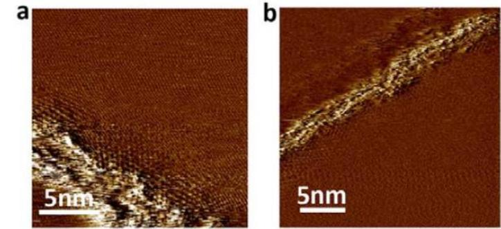
Figure S3| **a**, STM image of the mechanically cleavage edges of graphene; **b**, STM image of the oxygen-plasma etched edges of graphene.
