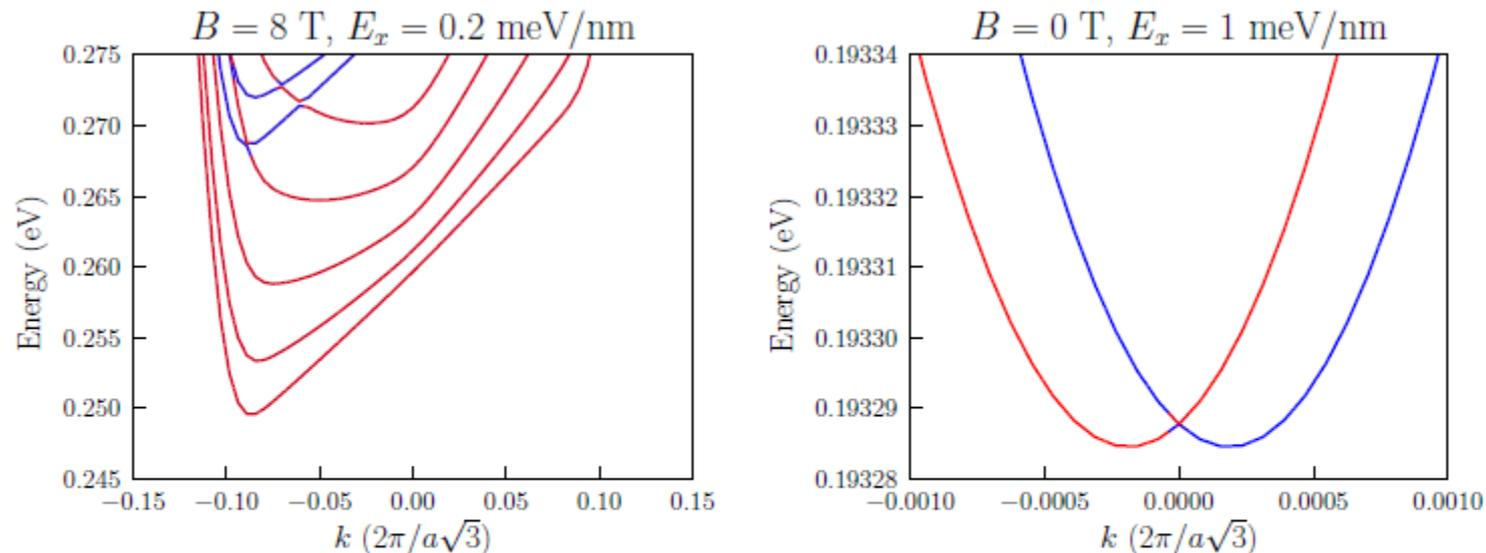
Figure S6: (left) Band structure of a 160 nm diameter hexagonal InSb NW in a magnetic field  $B = 8 \text{ T}$  (along  $(\mathbf{y} + \mathbf{z})/\sqrt{2}$ ), and in an electric field  $E_x = 0.2 \text{ meV/nm}$ . (right) Band structure of 160 nm diameter hexagonal InSb NW at  $B = 0 \text{ T}$ , in an electric field  $E_x = 1 \text{ meV/nm}$  (close-up on the lowest subbands, showing the effects of spin-orbit coupling).
