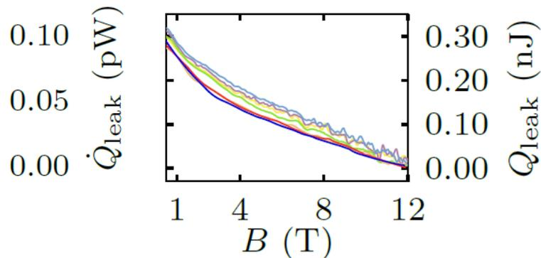
Parasitic heat leak inside the In island
