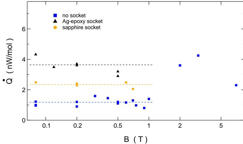
FIG. S5. The static heat leak  $\dot{Q}$  measured with MFFT for various magnetic fields and for three different socket designs: no socket, Ag-epoxy socket and sapphire socket. The dashed lines are guides for the eyes
