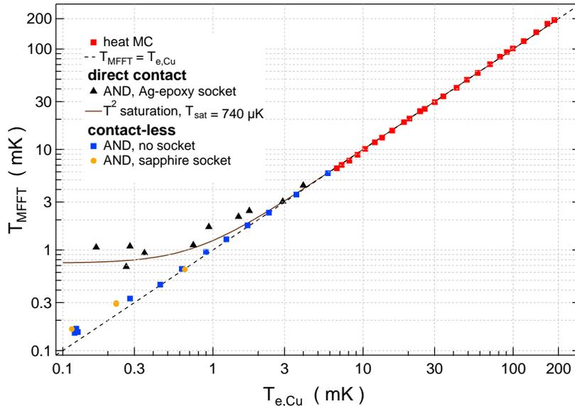
FIG. S6. Temperature measured by MFFT versus the temperature of the nuclear stage  $T_{\text{Cu}}$  with  $T_{\text{Cu}}$  extracted as in Fig. 4 of the main text. We compare two different gradiometer designs: old design with Ag-epoxy socket and improved design realized for no socket and sapphire socket.
