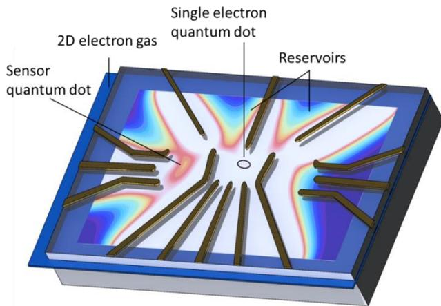
By applying voltages on nanofabricated surface-gates, a single electron quantum dot is imprinted into a two dimensional electron gas. The spin of this object is used for quantum computation.
