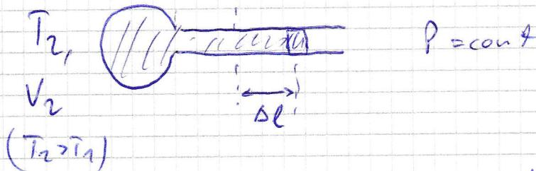
$\Delta V = A \cdot \Delta L$ ,  $A$  cross section of glass tube
