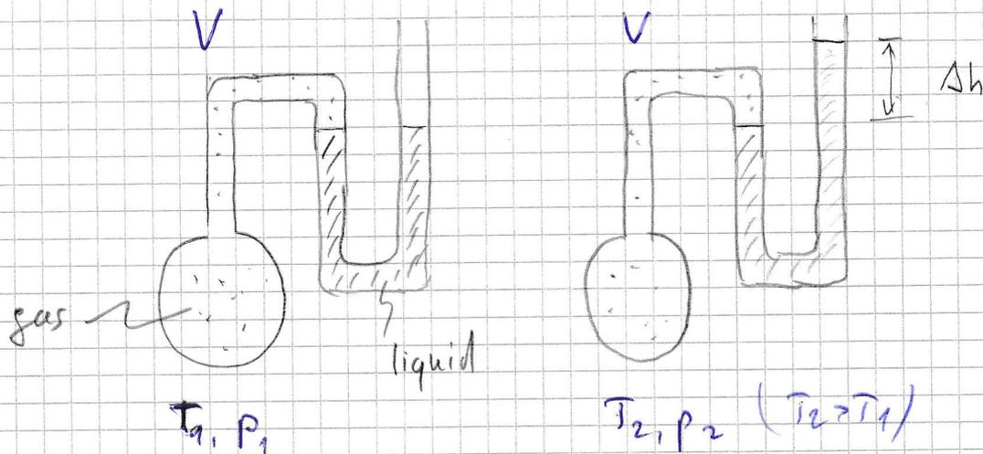
Total gas volume  $\sim$  const ( $V$ ) (gas container with larger volume than capillary tubes)
