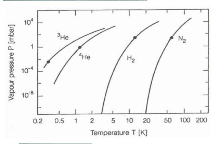
pumping on  ${}^{4}\text{He:} \sim 1 \text{ K}$  pumping on  ${}^{3}\text{He:} \sim 0.25 \text{ K}$
