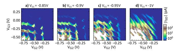
Fig. S3. Charge stability diagrams for different values of voltage applied to the central nanogate G1. By decreasing  $V_{\rm G1}$  the inter-dot tunnel coupling is increased, as evident from the transition from a double quantum dot (a) to a more single-dot-like configuration (d). Data were taken at  $V_{\rm SD} = -5\,\mathrm{mV}$  and  $V_{\rm L1,L2} = -4.5\,\mathrm{V}$ .
