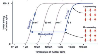
transferring this cooling via the chip's electrical contacts. This versatile and adaptable technique has been demonstrated in combination with modern cryogen-free refrigerators and successfully cooled 16 demagnetised measurement wires to fractions of a mK [5].
