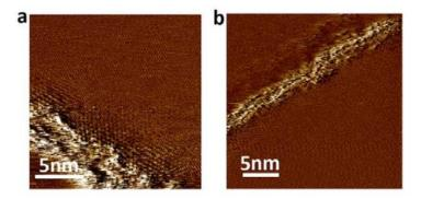
**Figure S3** | **a**, STM image of the mechanically cleavage edges of graphene; **b**, STM image of the oxygen-plasma etched edges of graphene.
