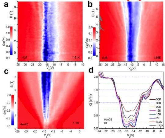
Figure S2| Magneto-transport measurements of other Z-GNR devices. a, sample# t127,  $l \sim 525$  nm,  $w \sim 60$  nm. b, sample#t128,  $l \sim 471$  nm,  $w \sim 101$  nm. c, sample# $dw \sim 28$ ,  $l \sim 500$  nm,  $w \sim 120$  nm. d, Temperature-dependent magneto-transport measurement of sampel# $dw \sim 28$  at B=9 T.
