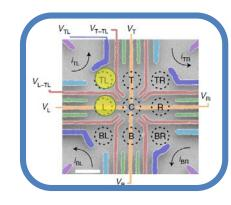
The spin mixing area (white/yellow) correspond to weakly tunnel coupled dots (or to S(2,0) and  $T_{+}(1,1)$  mixing)
