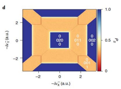
The high  $P_s$  probability area (blue) correspond to transfer the 2 electrons in another dot, preserving the singlet state. The mixing area (red) are where the electrons are split in 2 dots (and we have a mixture of S(1,1) and T<sub>0</sub>(1,1)
