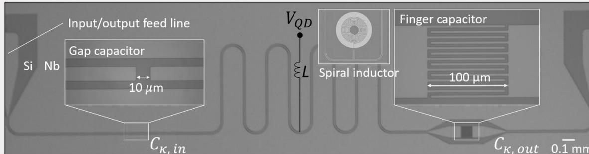
$f \sim 7\text{GHz} \sim 29 \mu\text{eV} \sim 330 \text{ mK}$ , resonator length  $\sim 8.5 \text{ mm}$
