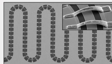
Height  $4 \mu\text{m}$ , length  $25\text{-}100 \mu\text{m}$ , width  $10\text{-}300 \mu\text{m}$
